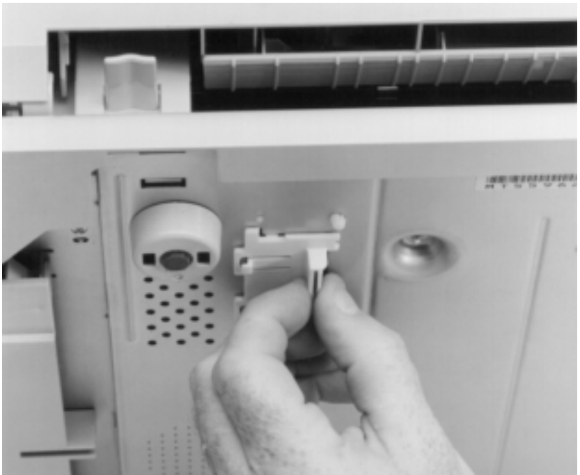
Figure 75. Engine test switch location
