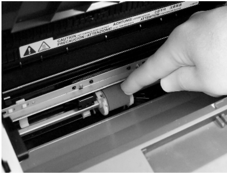
Figure 6-27 Remove the device pickup roller (5 of 5)
