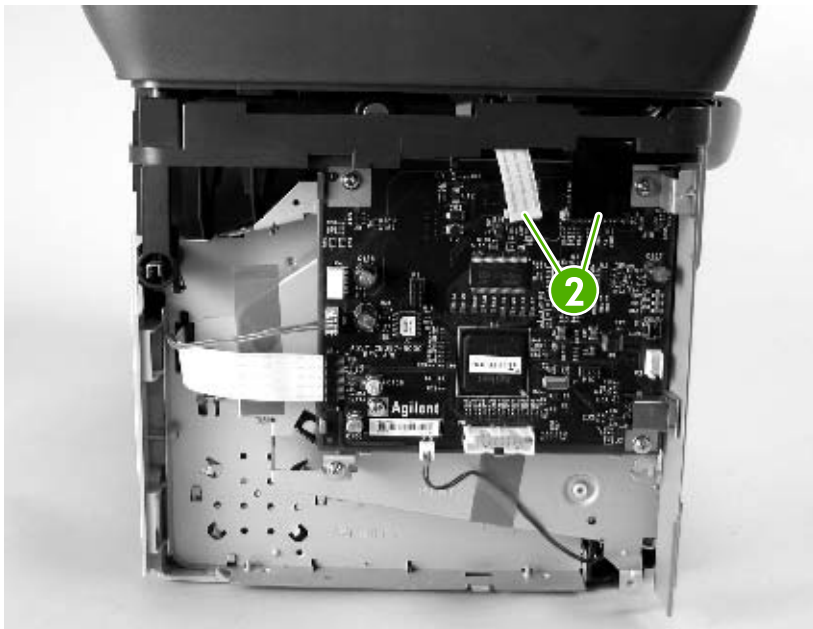
Figure 6-11 Remove the scanner assembly (4 of 11)
