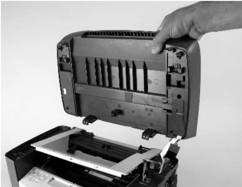
Figure 6-18 Remove the scanner assembly (11 of 11)
