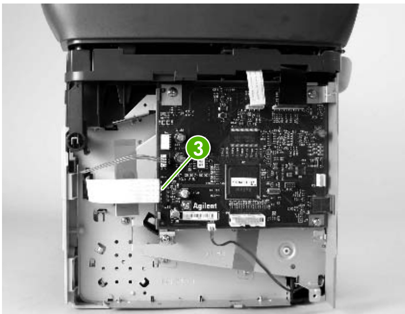
Figure 6-58 Remove the ECU (3 of 6)
