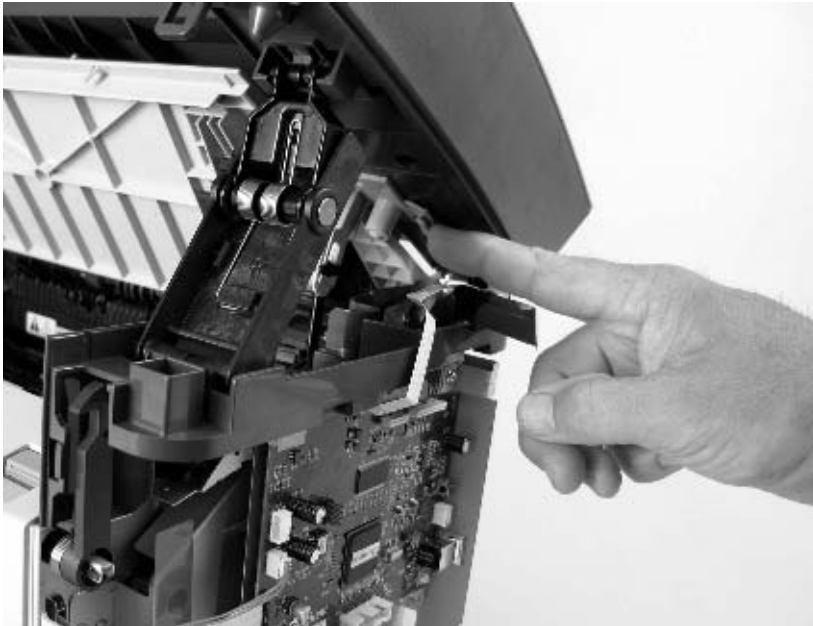
Figure 6-14 Remove the scanner assembly (7 of 11)
