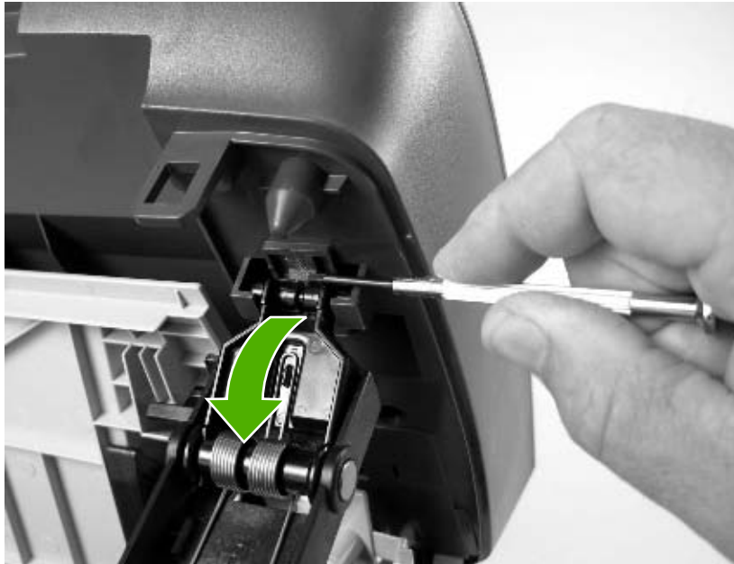
Figure 6-16 Remove the scanner assembly (9 of 11)
