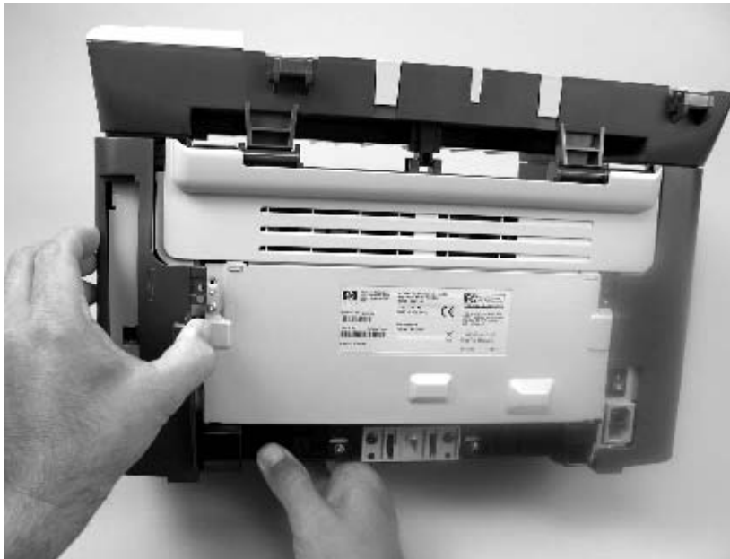
Figure 6-9 Remove the scanner assembly (2 of 11)
