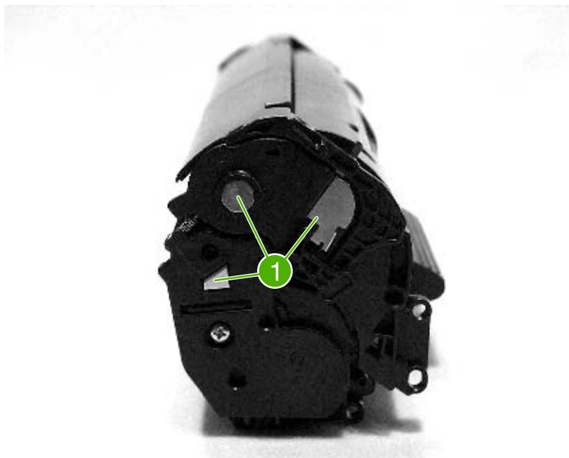
Figure 7-7 Print-cartridge high-voltage contacts
