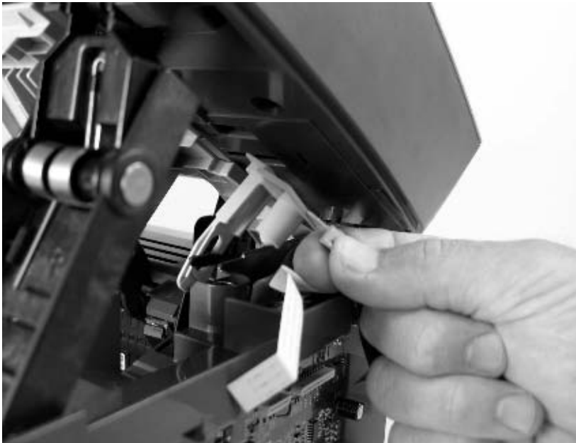
Figure 6-15 Remove the scanner assembly (8 of 11)
