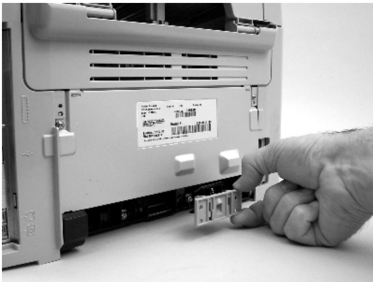
Figure 6-20 Remove the device separation pad (2 of 2)
