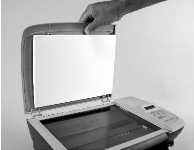
Figure 6-2 Remove the flatbed lid (1 of 2)
