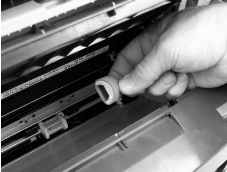
Figure 6-25 Remove the device pickup roller (3 of 5)
