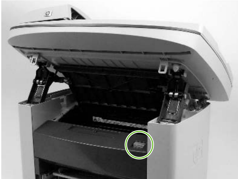
Figure 6-21 Remove the print cartridge (1 of 2)
