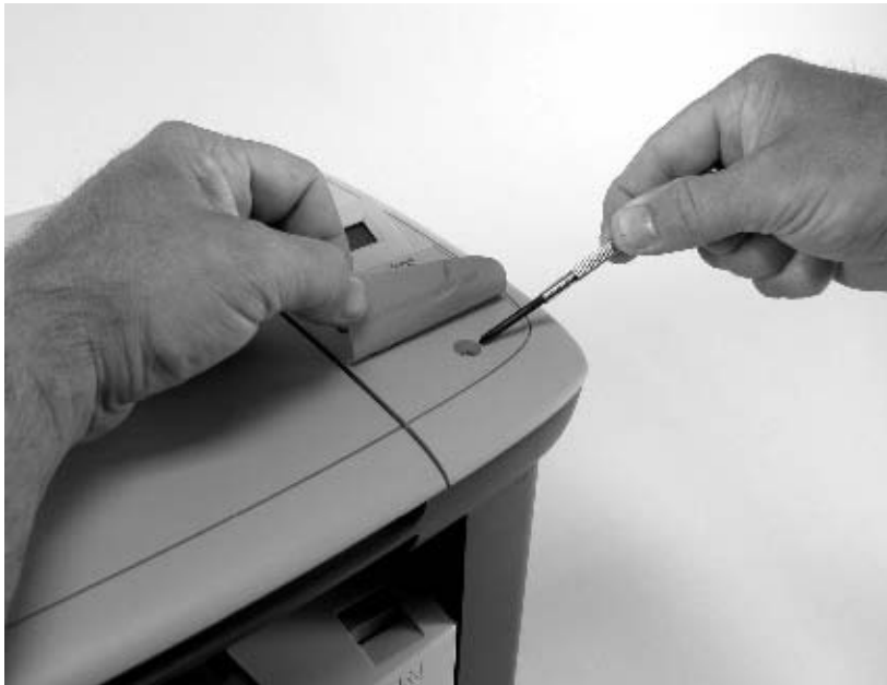
Figure 6-4 Remove the control panel (1 of 4)
