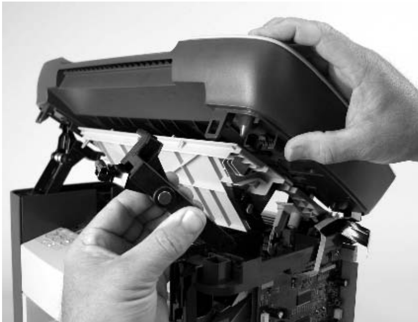
Figure 6-17 Remove the scanner assembly (10 of 11)
